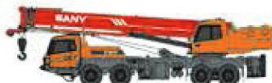
STC300H Maximum Load Capacity: 30t Telescopic Boom: 5 Sections, 10.5-39.5m
