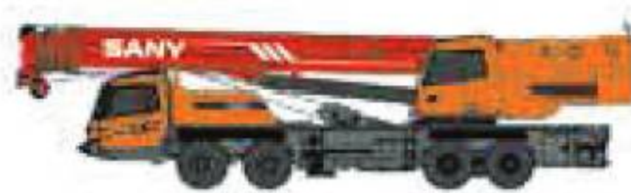
STC600 Maximum Load Capacity: 60t Telescopic Boom: 5 Sections, 11.5-43m
