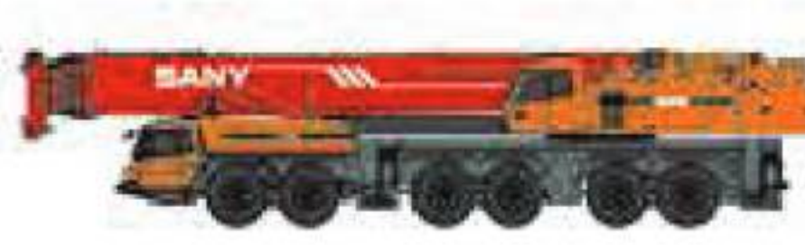
SAC3500 Maximum Load Capacity: 350t Telescopic Boom: 8 Sections, 15.2-70m
