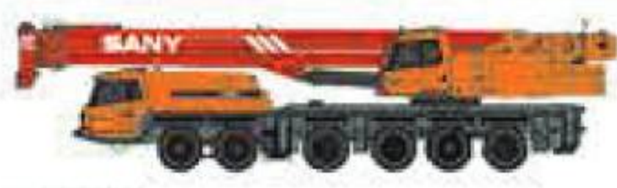
STC1000 Maximum Load Capacity: 100t Telescopic Boom: 5 Sections, 13.5-52m
