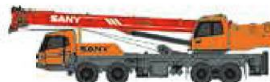
STC300TH Maximum Load Capacity: 30t Telescopic Boom: 4 Sections, 10.6-33.5m
