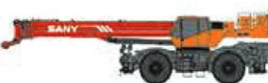
SRC550H Maximum Load Capacity: 55t Telescopic Boom: 5 Sections, 11.5-42.5m
