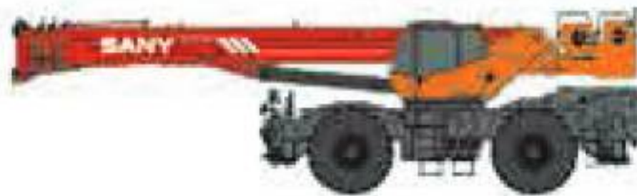
SRC550 Maximum Load Capacity: 55t Telescopic Boom: 4 Sections, 11.25-34.5m
