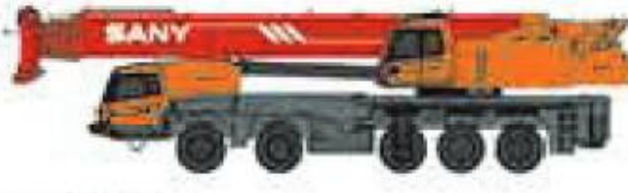
STC1300C Maximum Load Capacity: 130t Telescopic Boom: 6 Sections, 13.3-60m
