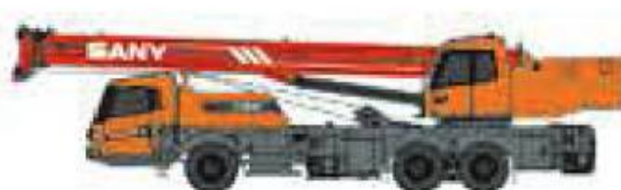
STC250 Maximum Load Capacity: 25t Telescopic Boom: 4 Sections, 10.65-33.5m
