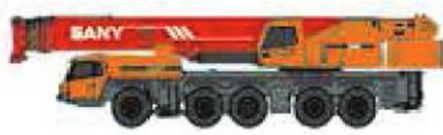
SAC2200 Maximum Load Capacity: 220t Telescopic Boom: 6 Sections, 13.5-62m
