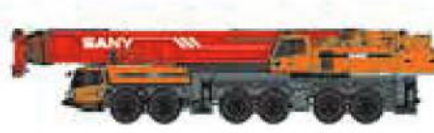
SAC3000 Maximum Load Capacity: 300t Telescopic Boom: 7 Sections, 15.4-80m
